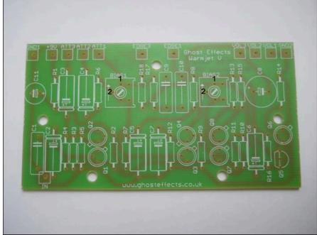
If you want to use internal trimpots then the board is designed to accommodate 2 different types of
